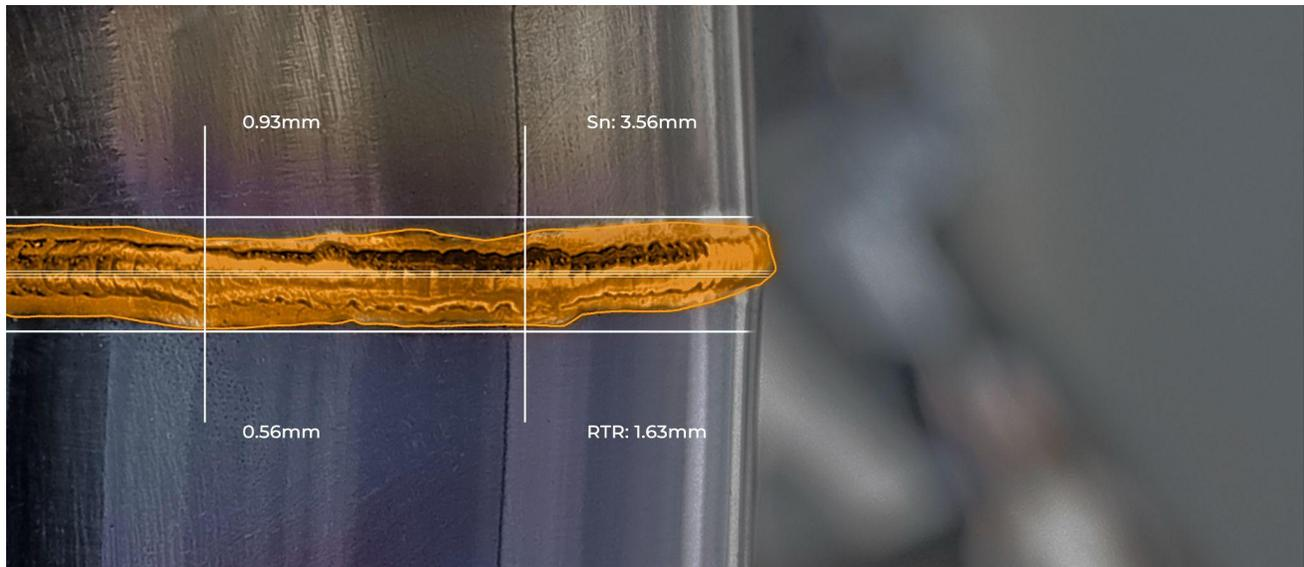
Deep learning based segmentation algorithms perform critical measurements with high accuracy for various weld seam types.
